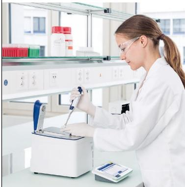
FastTrack UV/Vis technology guarantees that the instrument is ready at all times. No warm up time is needed for the Xenon flash lamp to reach stability, which speeds up measuring time. As the lamp is only used for real measurements, its lifetime is greatly increased.
