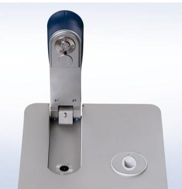
Micro-volume UV/Vis measurement is the method of choice if small sample amounts or if high absorption samples need to be measured. Only 1 µL of sample is required for reliable measurements. The pure sample is pipetted on the measurement surface and the arm is automatically locked to a precisely defined pathlength. Measurement errors are avoided as the sample does not need to be diluted.
