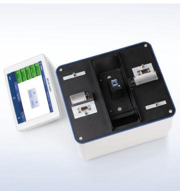
Exceptional ruggedness and reliability, thanks to the lack of moving parts in the optical section, long-lasting Xenon flash lamp and state-of-the art optical fibers. Their flexible connectivity to printers, PC, storage devices and barcode scanners, makes UV/VIS Excellence instruments a sound, sustainable investment for the future.
