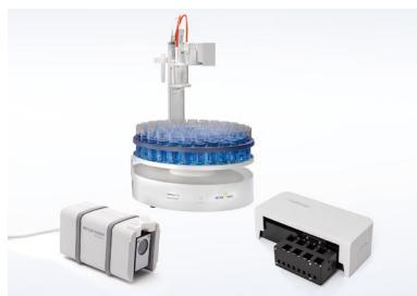
**CuvetteChanger:** Up to 8 cuvettes, thermostatable.
