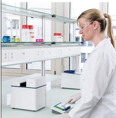
The CertiRef™ allows to quickly and easily verify the performance of the UV5Bio. It automatically verifies the resolution, photometric and wavelength accuracy, and stray light. Certified reference materials traceable to NIST are used and a comprehensive report documents all results. Performance verification has never been so easy, efficient and secure.
