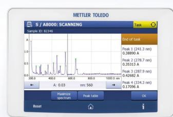
The user interface is intuitive and ensures efficient handling. With a large crisp touchscreen and clever usage of colors, spectra and results are clearly represented. For a closer look, pinching or stretching with two fingers on the touchscreen quickly zooms in on spectrum details, even when wearing protective gloves.
